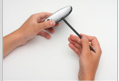
Using a spudger, gently pry apart the back case from the front case. It is easier to start on a side and work your way around the device.
