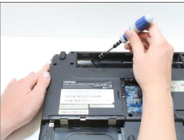
• Remove the three 3mm Phillips #1 screws inside the battery compartment.
