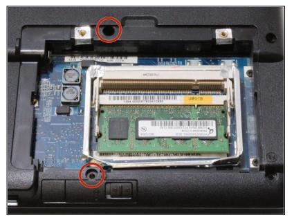
Unscrew the two 8mm Phillips #1 screws inside the RAM compartment.
