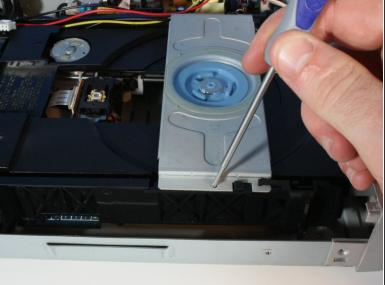
Remove the 6.3mm screws keeping the disc tray bracket connected to the disc tray.
