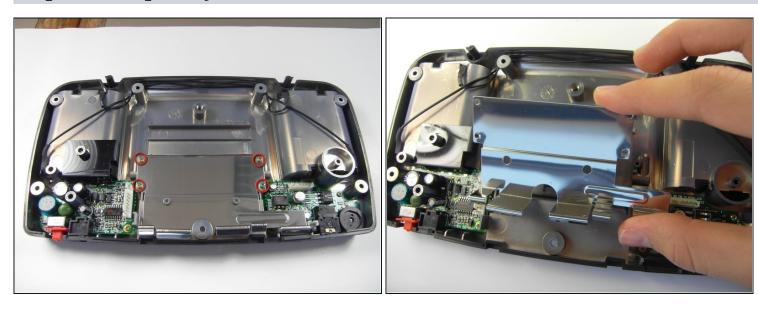
Unscrew the screws to remove the metal covering.
