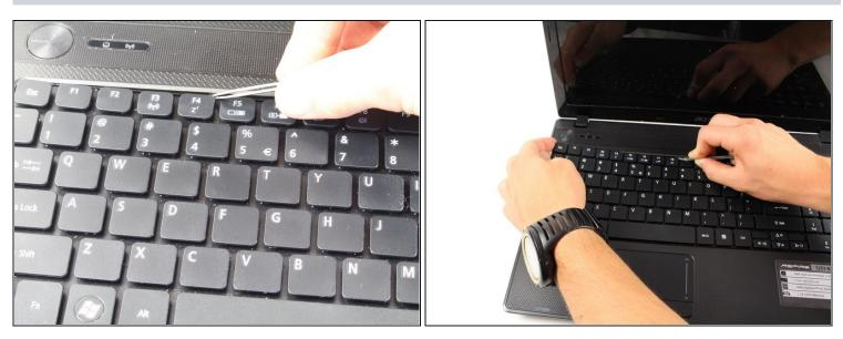
• Using thin tweezers push the tabs in the keyboard in and pull up on the edge of the keyboard.
