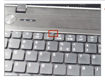
• Locate the tabs keeping the keyboard in place.
