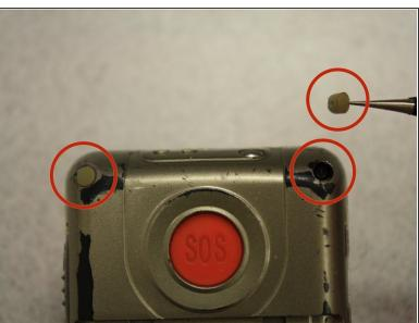
Remove the four rubber inserts from the screw holes using a pair of tweezers.
