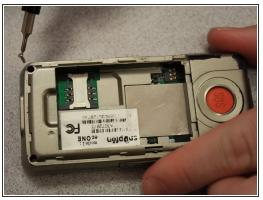
Remove the four 3.1mm screws in the corners with a Phillips #00 screwdriver.
