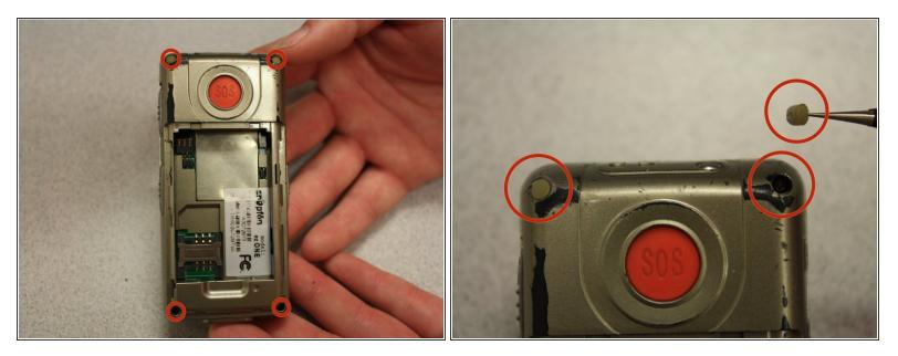
• Remove the four rubber inserts from the screw holes using a pair of tweezers.
