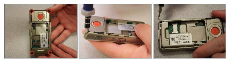
• Remove the four 3.1mm screws in the corners with a Phillips #00 screwdriver.
