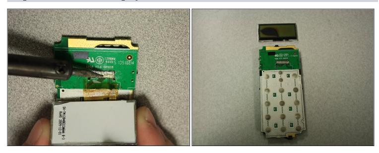
• Once you heat the solder connection, lightly tug the ribbon cable free. The LCD screen will be completely removed from the device.
