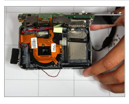
Slowly bend circuit board upwards (towards power button) until at 90 degree angle with remaining part of camera.
