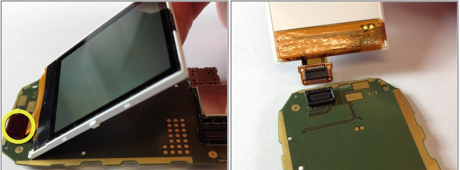
**⚠** Be gentle when pulling off the display screen. If pulled too hard, the orange connecting ribbon will rip.
