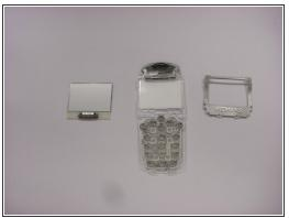
Once the metal frame is removed, the LCD display should fall from the keypad interface when tilted.
