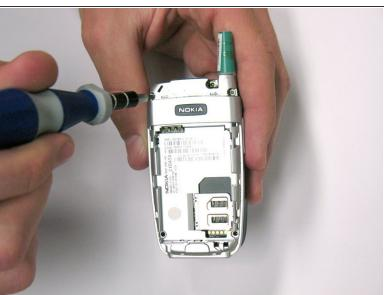
Remove the two newly revealed .208 inch screws at the top using a T-6 screwdriver.
