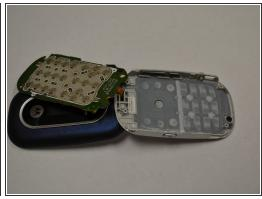
Using the plastic opening tool, gently lift the circuit board off of the four gray pegs that it rests upon.
