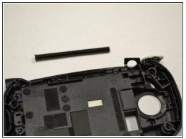
Using a plastic opening tool, lift and remove the antenna casing.
