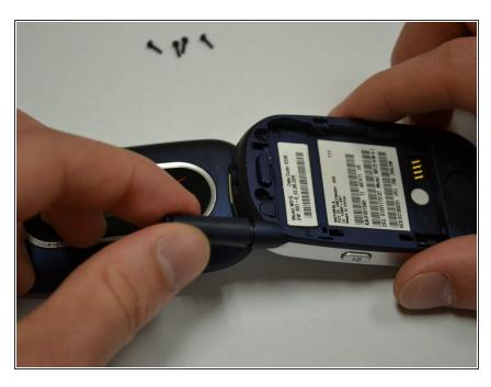
Gently twist the antenna in a counter-clockwise direction to unscrew it.
