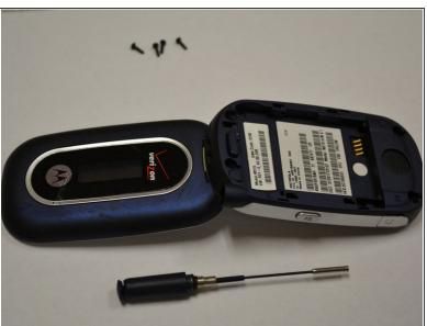
Pull the antenna out through the hole in the top of the frame and set it aside.
