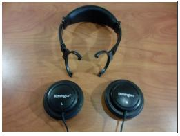
Repeat the process in Step 1 to remove the right speaker clamp.
