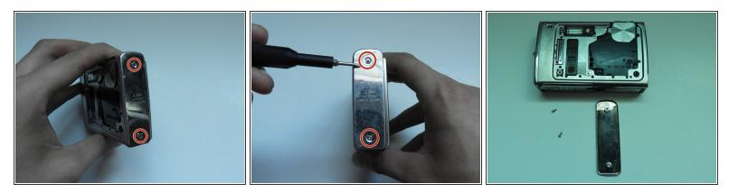
• Using the Phillips #00 screwdriver, unscrew the two screws on the side of the camera.
