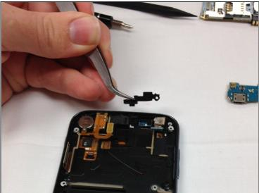
• Use the tweezers to remove the plastic bar which holds the camera in place.
