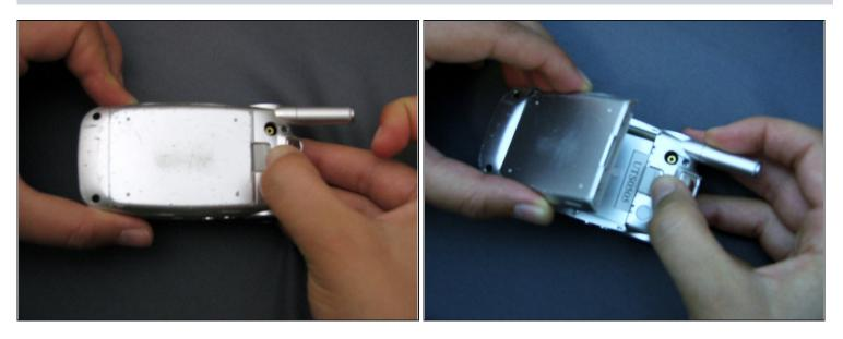
Hold the phone in one hand, slide the latch up, and pull the battery up to remove it.
