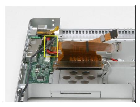
Disconnect the 4-pin power cable and orange ribbon from the DC/Sound card.
