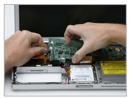
• Disconnect the DC-In connector from the left side of the logic board.
