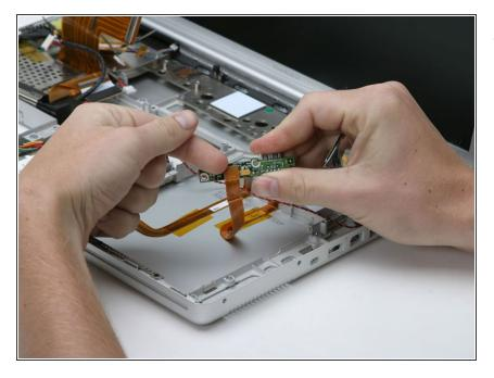
Lift the USB board up and disconnect the orange ribbon cable from beneath it.
