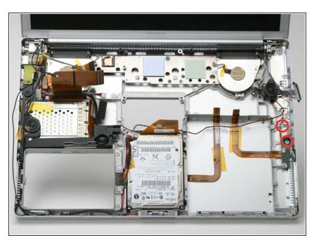
• Remove the two Phillips screws from the USB board.
