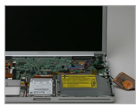
• Do not disconnect the PRAM battery from the logic board, but simply place it aside, allowing access to the optical drive.
