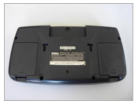
Place your device upside down and locate the two battery compartments.
