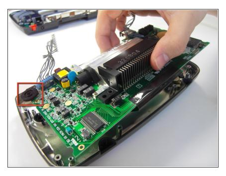
Slide the logic board out from under the circular black fastener at the topleft corner of the case.
