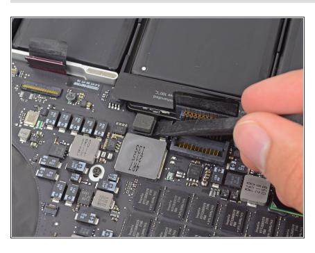
Use the flat end of a spudger to pry the trackpad ribbon cable connector up out of its socket.
