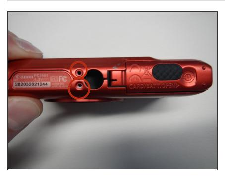
Remove the two screws on the bottom of the camera located near the battery door (Phillips #00 screwdriver) (4.0 mm).
