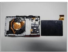
• Insert the flat side of the spudger tool carefully on the top of the LCD screen and lift the screen free
