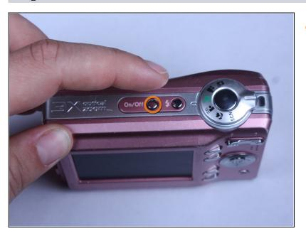
Turn the camera off by firmly pressing the power button located on top of the camera.
