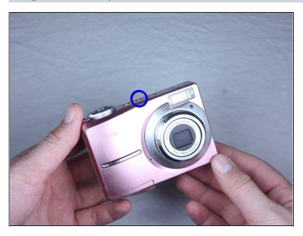
Turn off camera by firmly pressing the power button that is located on the top of the camera near the selector dial.
