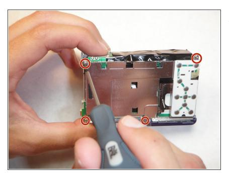
• Using the Phillips #00 screwdriver, remove the four screws on the outer edge of the LCD holding plate.
