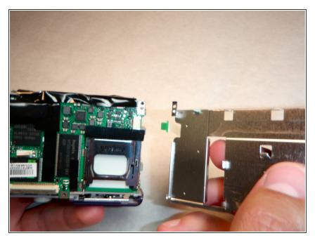
Remove the ribbon cable from its slot by gently pulling the LCD holding plate to the right.
