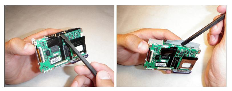
Do not touch ANY part of the logic board previously covered by the black film until the capacitor has been completely discharged. This camera has a 330V, 100 μF capacitor which can cause painful electric shock.
