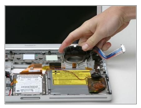
• Lift the fan from the front, and pull it out of the computer.
