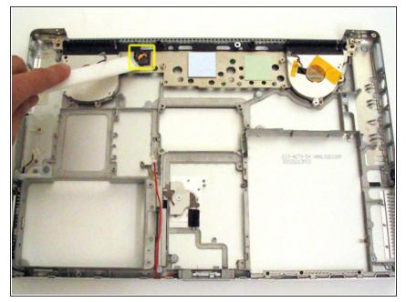
• Use a firm plastic edge to scrape the thermal material off the heat sink.
