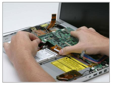
Disconnect the battery cable from the front, left corner of the logic board.
