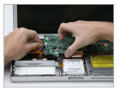
• Disconnect the DC-In connector from the left side of the logic board.
