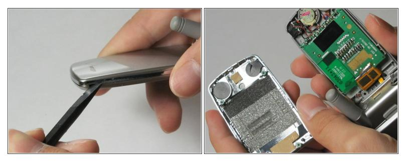
• Locate the small gap at the top right corner of the phone as shown. Use the spudger to gently pry the back casing off.
