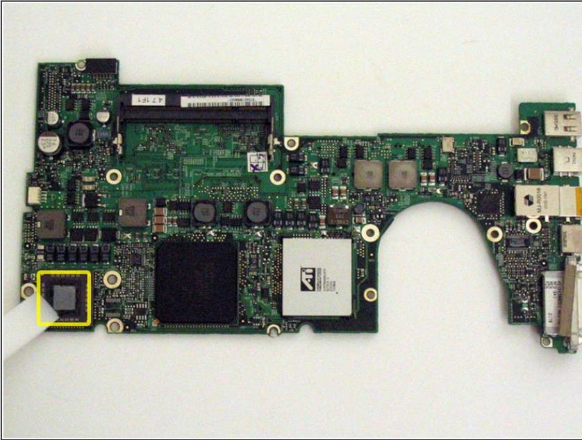
✦ Important: when you reinstall a logic board, you'll need to replace the thermal paste that goes between the processor on the logic board and the heat sink. Failure to remove the old paste and apply a new layer can cause the computer to overheat and sustain damage. The following steps refer to replacing the thermal paste between the processor and heat sink; follow these steps only when you are ready to place the logic board in the computer.
