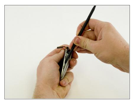
Carefully pry apart the casing with the spudger tool.
