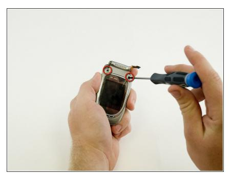
Remove screws with #0 Phillips screwdriver.
