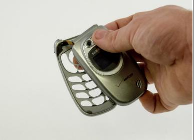
• When using a spudger the keypad housing comes off quite easily, although it may be necessary to guide the ribbon cable through the slot in the housing.
