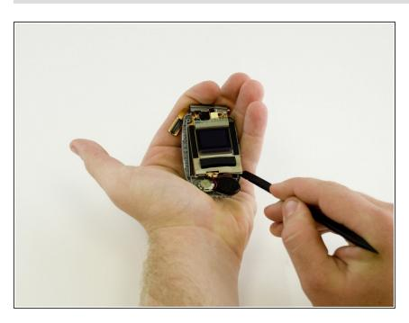
Carefully pry off the screen with the spudger.
