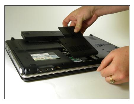
Remove the memory module compartment cover.
