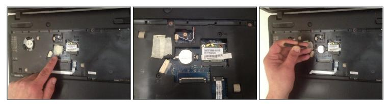
• This is the internal CMOS / BIOS battery. Use small screwdriver to remove it.
