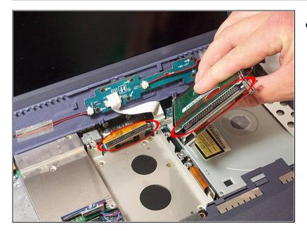
Slowly pull the hard drive away from the ribbon by holding the plastic connector at the end of the ribbon and pulling on the Hard Drive. The Hard Drive should now be completely free of the laptop and the two connecting ends displayed in the picture should be visible.
