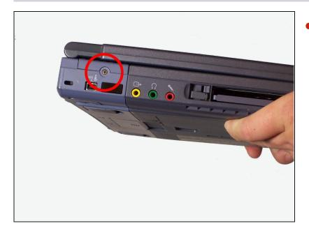
Use your Philips #00 screwdriver to unscrew the small screw counterclockwise. This screw is for the audio/visual jacks on the left side of the laptop.
