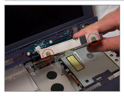
• The hard drive is attached to the metal outer case by four screws, two on each side.
