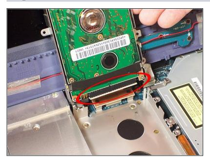
The Hard Drive box is now unfastened. You can free it from the laptop by pulling up, but be careful because it is held in place by the surrounding metal pieces so a little strength, yet care, is needed. When free, do not immediately remove it, there is a ribbon cable connecting it to the laptop.
