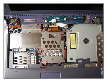
• The hard drive is the metal box in the middle. Use your Philips Head screwdriver to remove the four screws that attach the cage to the motherboard.
