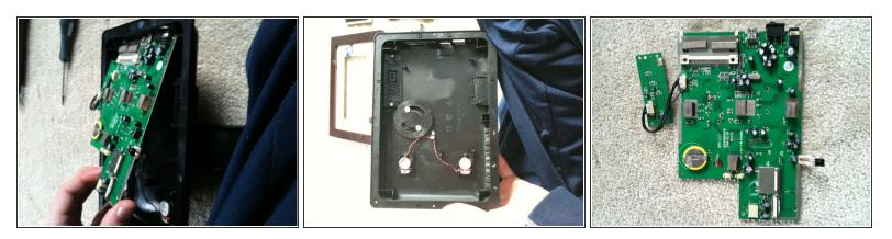
• Remove the logic board, and the case and speakers remain.
