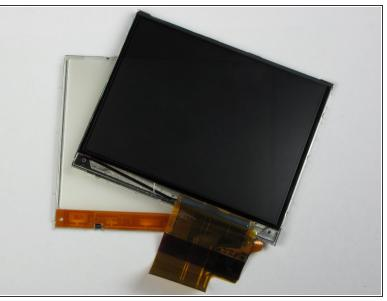
(i) The display consists of two screens which are held together by the ribbon.
