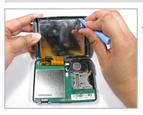
Apply pressure to the tabs holding the screen in place with the plastic opening tool
