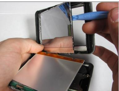
Apply pressure to the same tabs again to remove the front of the screen.
