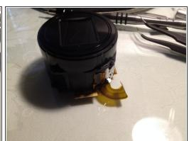
• The lens assembly is now removed from the body.
