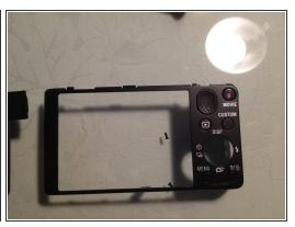
Gently pull the frame off the LCD screen, outwards and upwards from the bottom of the camera and remove it.
