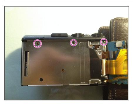
Remove the three screws. Gently use a spudger to lever/remove the metal assembly away from the camera body and place it aside.
