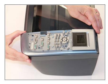
• From the front of the printer, remove the button panel by pulling it towards you while slightly lifting it up.
