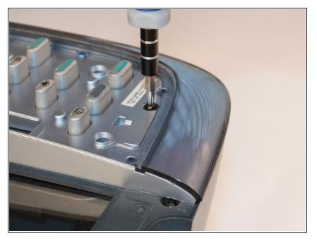
• Use a T9 Torx screwdriver to remove the 9 mm screw.
