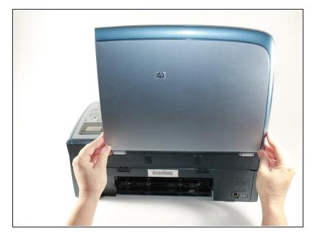
With two hands, grasp the lid on both sides near the hinges and lift straight up to release the lid from each hinge.
