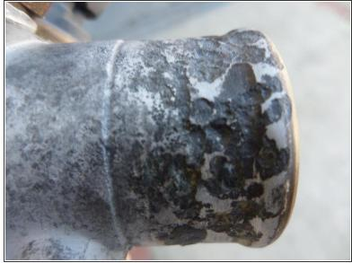
• If, after sanding, you find that the necks on your housing are severely pitted you may consider fixing them with a light coat of epoxy to fill the pits. If this doesn't work you may need to source a good used part, or a new housing.
