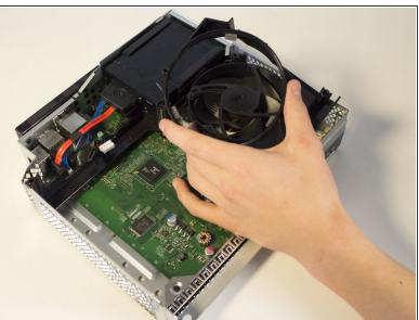
Flip the Xbox over and take out the heat sink plastic shield.
