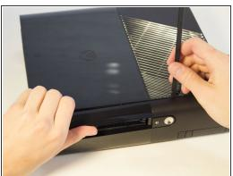
Beginning on the left side without the grate, run the spudger along the crevice until you've reached the grated part, while holding the part that's being separated as you go.
