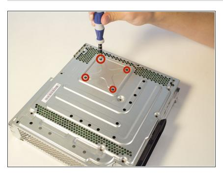
Flip the Xbox to the back and take your T10 torx screwdriver and take out the last four 6 mm screws labelled A1-4.
