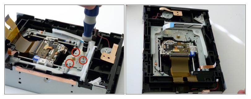
Now you can see the inside of the optical drive. The motor is held in by three small 5mm silver screws. Remove them.
