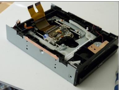
Lift up the motor and replace it with a new one. Now you just need to put it back together!
