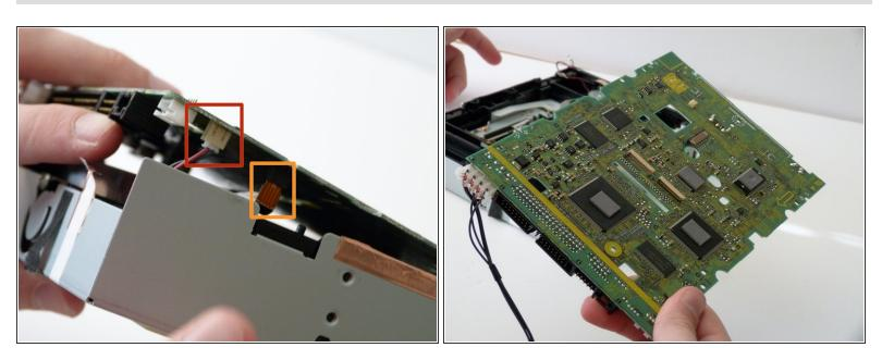
Slowly lift up the circuit board. Make sure to disconnect the connector and ribbon cable on the underside of the circuit board before fulling removing it.
