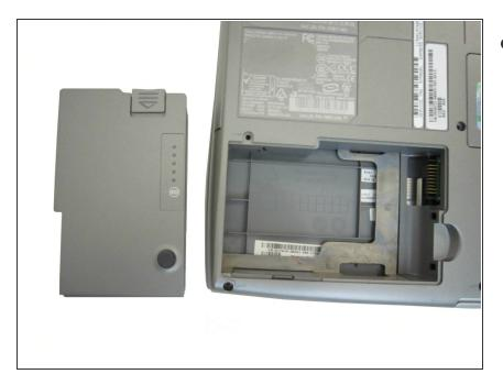
Remove the battery from its compartment.
