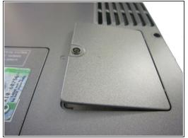
• Remove the 3.9mm screw with a Philips #1 screwdriver containing the modem.
