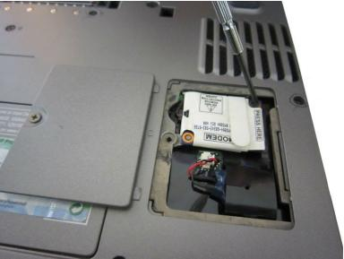
Remove the 3.9mm Philips #1 screw on top of the modem.
