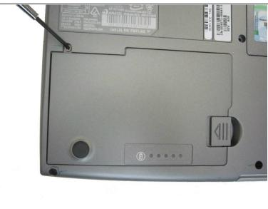
• Remove the 3.9 mm Phillips #1 screw from the battery compartment.
