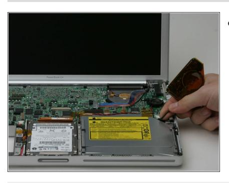
Disconnect the PRAM battery cable from the logic board and pull the PRAM battery out.
