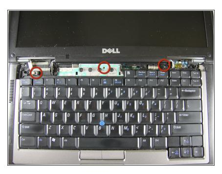
Unscrew the top portion of the keyboard using a #00 screwdriver
