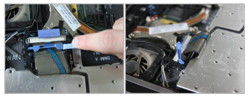
Using a small spudger, pull back on the black bar to release the blue lever
