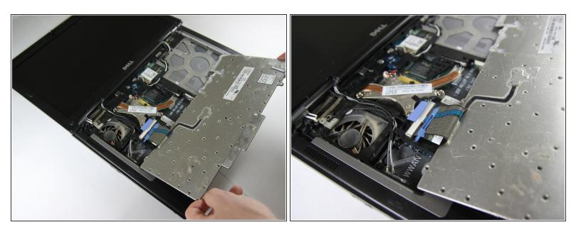
Once keyboard is out of the case, lay it face-down on the track pad
