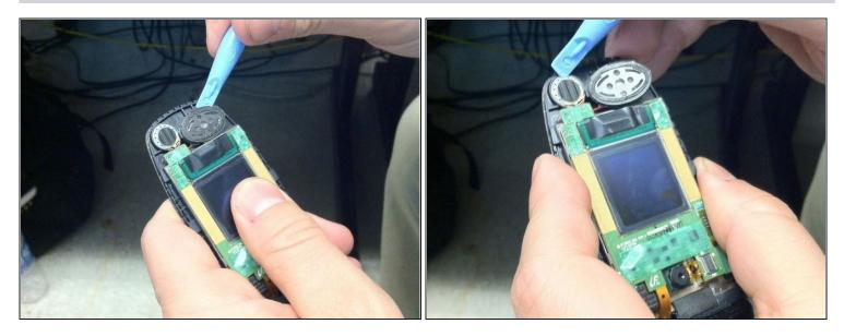
• Using a plastic opening tool, pry the speakers from the case. These are located at the top of the back of the phone.
