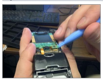
Using a plastic opening tool, disconnect the electrical connector. The electrical connector is located near the hinge and is revealed when the front cover is removed.
