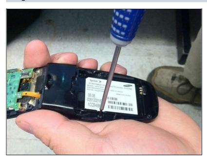
Using a #00 Phillips screwdriver, remove four screws from the bottom half of the phone in the battery compartment. The screws are in each corner. Place screws off to the side.
