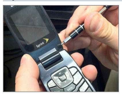
Peel off the screw covers and remove two exposed Phillips head screws with a small Phillips head screwdriver.
