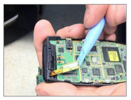
Once the back is removed, use a plastic opening tool to disconnect the electrical connector near the hinge.
