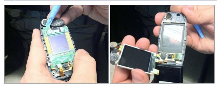
• Using a plastic opening tool, lift the screen assembly from the case.
