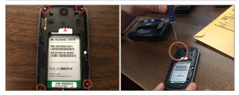
• Using the Phillips #00 Screwdriver, take out the four small screws located at the four corners of the phone.
