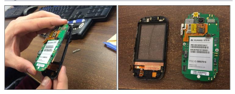
• Once the silver and orange tabs are pulled back, carefully pull the motherboard apart from the front case.
