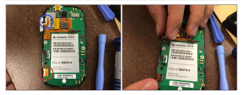
• To remove front case from the motherboard, first pull back the silver tab (highlighted in blue) and the orange tab (highlighted in red).
