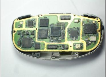
Holding the phone with the screen facing you, remove the top half of the phone from the circuit board.
