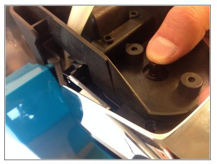
• Push down lightly on the nozzle that the hose was attached to. The plastic housing along with the needle should pop off without much force.
