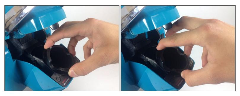
• Firmly rock the K-cup holder from side to side, loosening the K-cup holder from its seat.
