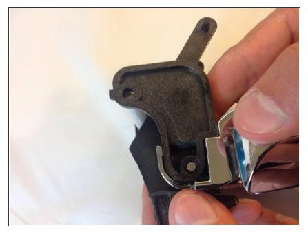
• Once the both snap rings are removed, pull on the plastic side plates to remove them. It shouldn't take much force to remove them.
