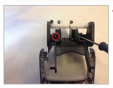
Unscrew the two 9mm #1 Philips screws from the handle assembly.
