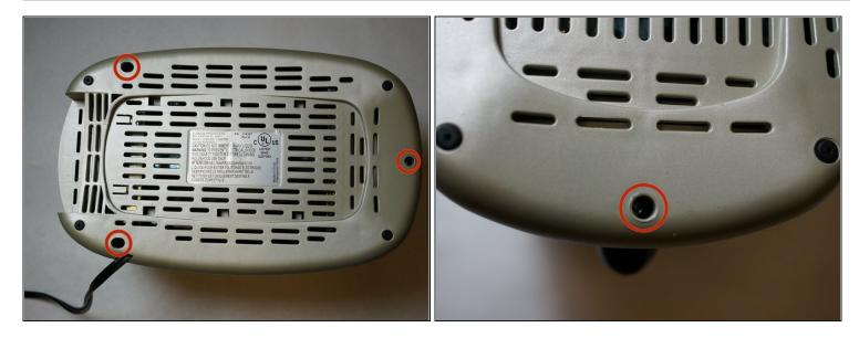
• Using the Phillips-head #2 screwdriver, unscrew the three 1cm Phillips-head screws on the plastic base of the toaster to separate the outer metal shell from the plastic base.
