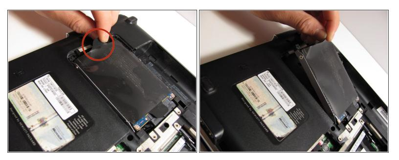
• Use the Mylar tab to lift the hard drive up, and then slide out to release it from the hard drive bay.
