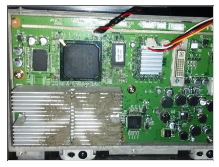
now we need to remove the heatsink from the board. there are two screws, they're spring loaded, number two phillips screw driver to remove them and the heatsink should lift off.
