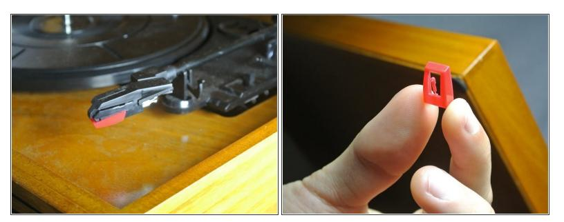
The needle is the red plastic piece on the end of the arm. The needle snugly fits over the lower portion of the head, or front end, of the arm.
